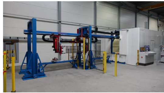
Pic. 3: System for welding different towel radiators
